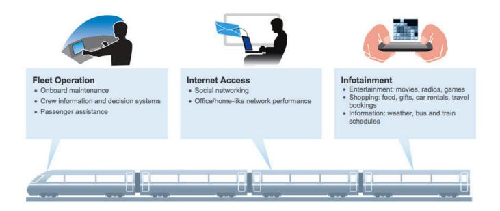
Delivering smooth Wi-Fi access is critical for onboard rail networks. Onboard environments have limited space and are prone to severe vibrations, making it more difficult to design a good Wi-Fi network, and requiring wireless devices tailor-made to ensure system stability. In addition, wireless devices that are used onboard must be able to ensure that every passenger has enough bandwidth and secure network access, without having to worry about being hacked.
