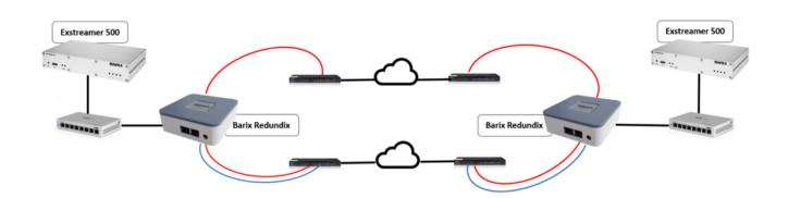
Redundix by Barix is a solution that improves the quality of an RTP stream link using two mechanisms. The first is time-diverse routing, where the same audio stream is sent twice over the same link, immediately on encoding, and also time-delayed. The second is path divergent routing, where two streams are sent using separate networks.
