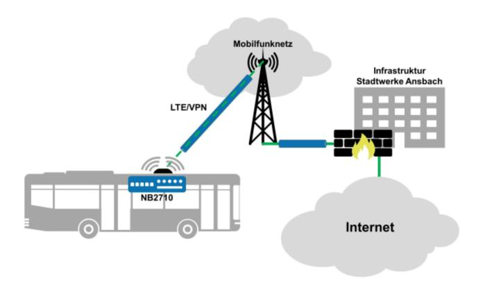
For the communication over the mobile network, Stadtwerke Ansbach uses two SIM cards. One serves exclusively for the passenger WiFi and the second for various other IT applications such as passenger counting. This leads to a clear separation of passenger and operating data and also a specific billing gets easier.
